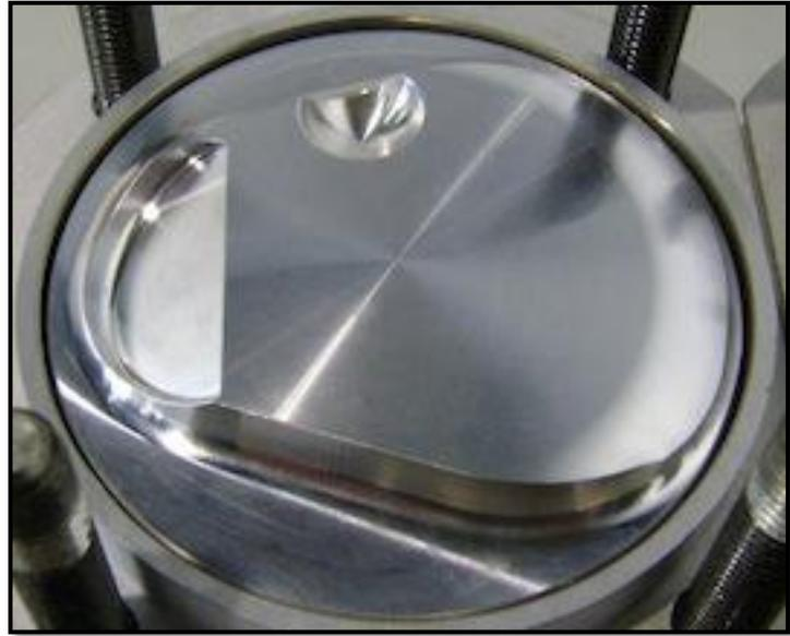
The stock 356 cylinder head has always suffered from poor flame travel, especially when the chambers are opened up for better flow. The larger chamber then requires a taller and heavier dome on the piston, which not only adds weight to the piston, but further inhibits flame travel across the top of the piston dome. Twin spark plugs solve this problem, but not everyone wants the non-original look of twin-plug ignition, and the added expense that comes along with it.
